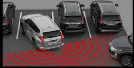
The driver is alerted when the rear radar sensors detect approaching vehicles nearby while the reverse gear is engaged. A warning message appears in the multi-information display, a buzzer sounds, and an indicator blinks in both side view mirrors. (GT 4WD)
