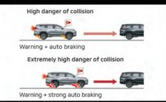
When there is a risk of collision, the FCM system alerts the driver with a visual and audible warning. If the driver does not respond, the system automatically applies moderate to emergency braking. (GT 4WD)
